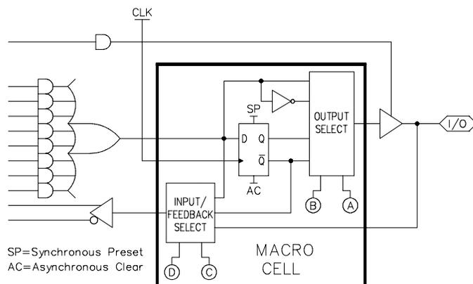
In addition to emulating the four PAL-type output structures (configurations 3, 4, 9, and 10), The macrocell provides eight additional configurations. Equivalent circuits for the twelve macrocell configurations are illustrated in Figure 22. These structures are accessed by specifying the PEEL™22CV10A+ or PEEL™22CV10A++ option when assembling the equations.
