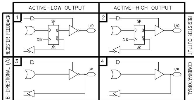
**Table 1. PEEL™22CV10A Macrocell Configuration Bits**
